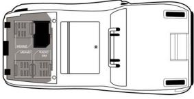
Figure 14 Installing MSAM Card
